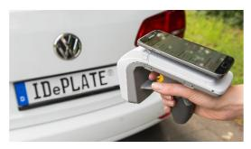
When paying contactless via card or smartphone, the data is transmitted via near-field communication (NFC). With the TÖNNJES identification system, scanning devices identify the secure number plates from a large distance. Integrated into the IDePLATE, as well as into the IDeSTIX, is a cryptographic chip containing a unique identification number. RFID makes it possible to
